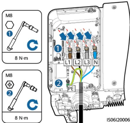
5. Tighten the thread-lock sealing nut.
