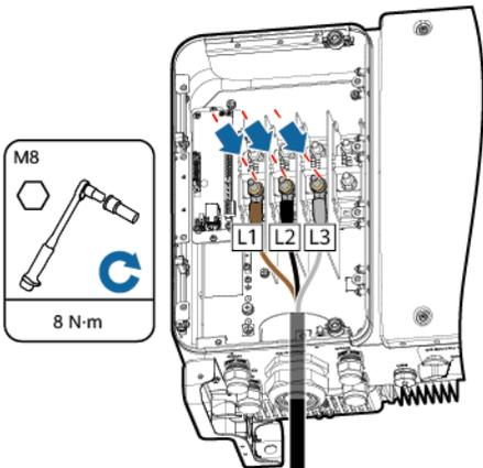
b. Four-core cable (including the ground cable but excluding the neutral wire)
