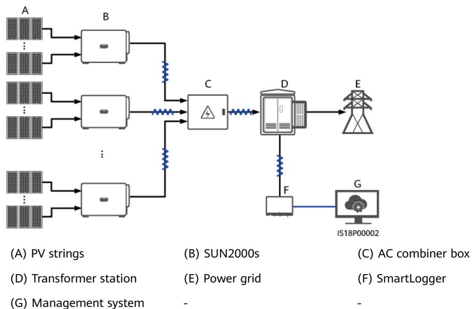
**Figure 5-2** MBUS networking application (double-column transformer +SmartMBUS CCO)
