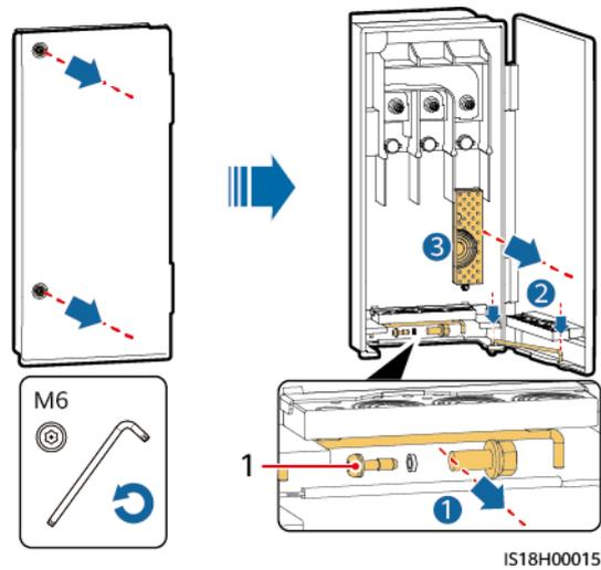
(1) Position for binding the ground screw
