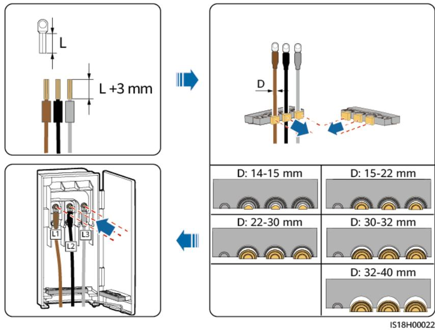
**Figure 5-13** Multi-core cable connection (using a three-core cable as an example)
