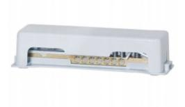
The potential equalization rail 7x25, 1x50, 30x4 is a device used to protect electrical installations and lightning protection systems from uncontrolled voltage surges. It is permanently mounted on a rail. The product includes one flat cable measuring  $30 \times 4$  mm, seven single or multi-wire cables with a cross-section of up to 25 mm<sup>2</sup>, and one round cable with a cross-section of 50 mm<sup>2</sup>.
