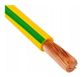
The H07V-K LGY cable with a cross-section of 6 mm2 and a voltage of 750V is an electrical wire with a yellow-green color, made of multi-stranded, flexible copper core, insulated with polyvinyl chloride (PVC). It is a low-voltage cable designed for wiring installations.
