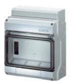
Small distribution boards for outdoor unprotected installations, such as the modular distribution board accommodating from 3 to 54 modules Model KV 8109, are ideal for applications requiring compact size and weather resistance. This particular distribution board is characterized by the absence of PE and N terminals, which is essential for the specific application and configuration of the installation.
