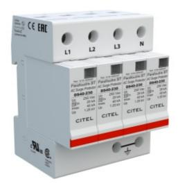
Surge protector for T2 AC networks - CITEL AC-DS44-230 operates at four discharge speeds with a current In = 20kA (8/20µs), utilizing a varistor block as the main protective element in each module. Designed for installation in low-voltage switchboards as the second stage of protection against induced surges. It is also available in a version with remote signaling capability (-S).
