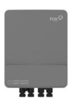
The fire safety switch FOXESS S-BOX is a device designed to control the supply of direct current from photovoltaic panels. It ensures safety by disconnecting the direct current circuit in case of a disruption in the supply of alternating current. It operates by connecting the DC circuit after the AC power is restored. This device is extremely useful in the event of a power grid failure or intentional disconnection of building power when there is a risk of fire.
