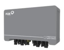
The fire safety switch FOXESS S-BOX-4 is a switch designed to control the supply of direct current from photovoltaic panels. It ensures safety by disconnecting the direct current circuit in case of interruption in the supply of alternating current. It operates by connecting the DC circuit after the AC power is restored. This device is extremely helpful in case of a power grid failure or intentional disconnection of building power when there is a fire risk.
