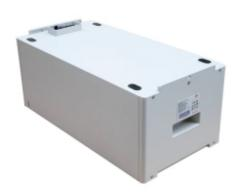
BYD BOX PREMIUM HVS BATTERY - high-voltage battery with Lithium-Iron-Phosphate cell technology. The BYD Premium HVS kit connects 2 to 5 series-connected battery modules. The usable capacity of the kit ranges from 5.12 kWh to 12.8 kWh. BYD HVS allows the creation of a direct connection of 3 sets of Battery-Box Premium HVS in a parallel arrangement, ensuring a maximum kit capacity of 38.4 kWh.
