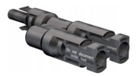
MC4 tee connector (socket) MC-PV-AZS4 for parallel connections Construction: 2x socket (+) KBT4... → plug (-) KST4
