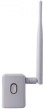
SolarEdge WFRPT-B-S1-RW is a wireless signal amplifier and gateway that enhances the Wi-Fi signal between the wireless gateway on the router and the inverter.
