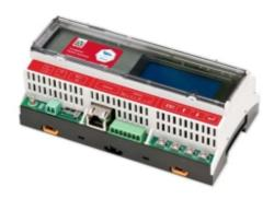
The SolarEdge SE1000-CCG-F-S1 fire gateway enables centralized management of SolarEdge system safety. With it, firefighters can swiftly halt energy production from SolarEdge solar installations using either a manual alarm switch or automatically through the fire control panel system. When energy production is stopped, the SafeDC $^{\text{TM}}$  feature reduces the string voltage to a safe level.
