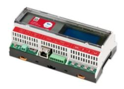
The SolarEdge SE1000-CCG-F-S1 fire gateway enables centralized management of SolarEdge system safety. With it, firefighters can swiftly halt energy production from SolarEdge solar installations using either a manual alarm switch or automatically through the fire control panel system. When energy production is stopped, the SafeDC $^{\text{TM}}$  feature reduces the string voltage to a safe level.
