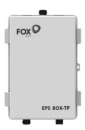
FoxESS EPS-Box TP is additional equipment that can be installed in FoxESS three-phase energy storage systems. The EPS BOX serves as an automatic disconnect for the local AC power grid and activates the EPS circuit for selected receivers, switching circuits to backup power provided by the EPS in the device. This device is fully maintenance-free and consists of two interlinked contactors enabling seamless switching of connected circuits.
