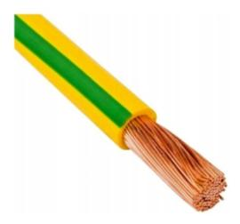
The H07V-K LGY cable with a cross-section of 16 mm2 and a voltage of 750V is an electrical wire with a yellow-green color, made of multi-stranded, flexible copper core, insulated with polyvinyl chloride (PVC). It is a low-voltage cable designed for wiring installations.
