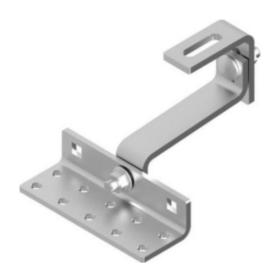
The VARIO roof hook with double adjustment, measuring 150 mm in length and made of Magnelis material, is an ideal solution for mounting on roofs covered with concrete or ceramic tiles. Thanks to its design and the use of innovative Magnelis material, this hook provides exceptional durability and resistance to weather conditions.
