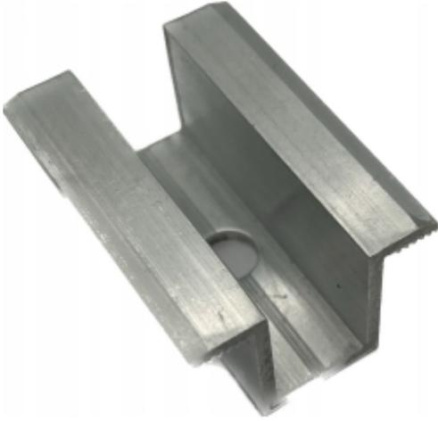
Anodized middle clamp. It is used for connecting and stabilizing photovoltaic modules while providing an aesthetic appearance. Dimensions: length: 50 mm height: 25 mm thickness: 3 mm color: silver Hole: M8
