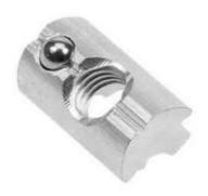
A sliding insert is a nut that enables a stable and secure connection of middle and end clamps to the profile. The ball located on the insert allows for proper stabilization and ease of positioning the clamp in the desired position on the mounting profile. Utilizing sliding inserts with balls for mounting photovoltaic panels significantly streamlines the installation process.
