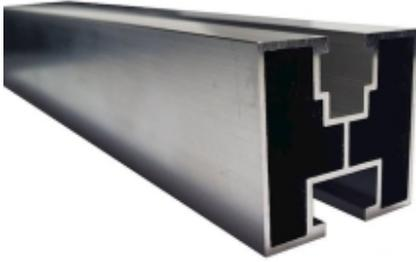
The aluminum profile 40x40 with a hexagonal screw, with dimensions L: 2200mm, is made of aluminum. Its main purpose is to enable the installation of photovoltaic panels using middle and end clamps.
