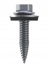
Sheet metal screw 6x25 stainless steel (Bi-metal) with EPDM washer Reisser - a bimetal screw for thin sheets. The sheet metal screw is used for fastening profiles and sheets to steel and aluminum structures. Useful for installing photovoltaic structures.
