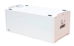
BYD BOX PREMIUM HVM BATTERY - high-voltage battery with Lithium-Iron-Phosphate cell technology. The BYD Premium HVM kit connects 3 to 8 series-connected battery modules. The usable capacity of the kit ranges from 8.3 kWh to 22.1 kWh. BYD HVM allows the creation of a direct connection of 3 sets of Battery-Box Premium HVM in a parallel arrangement, ensuring a maximum kit capacity of 66.2 kWh.
