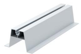
The trapezoidal bridge with EPDM gasket is designed for mounting photovoltaic panels on trapezoidal sheet metal. It features an aluminum rail and mounting profile measuring 70 mm x 300 mm. The EPDM gasket ensures a tight seal, protecting against moisture penetration. This bridge enables proper and stable installation of photovoltaic panels on roofs or other surfaces covered with trapezoidal sheet metal.
