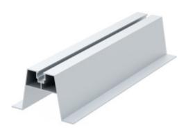
The trapezoidal bridge with EPDM gasket is designed for mounting photovoltaic panels on trapezoidal sheet metal. It features an aluminum rail and mounting profile measuring 70 mm x 300 mm. The EPDM gasket ensures a tight seal, protecting against moisture penetration. This bridge enables proper and stable installation of photovoltaic panels on roofs or other surfaces covered with trapezoidal sheet metal.
