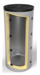
Buffer tank for black water, insulated, in OEM BLACK v2 200 G cover, without coil, with a capacity of 200 liters, is used for storing hot boiler water, which can then be used to supply thermal energy to the heating system (e.g., underfloor, wall-mounted, or radiators) when the furnace or boiler is not operating. It serves as a type of heat storage.
