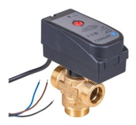
The 3-way valve for heat pumps 6-10 kW HP 3WV KAISAI is a switching device used in heating, cooling, and domestic hot water systems. It is installed to redirect flow between two different installations. Controlled by an SPST signal, it can be activated by any thermostat or switch. This valve is specifically designed for KAISAI heat pumps with a power range from 6 to 10 kW.
