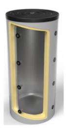
Buffer tank for hot water made of black steel, insulated, in OEM BLACK v2 300 G casing without coil, with a capacity of 300 liters, is used for storing hot boiler water, which can then be used to supply thermal energy to the heating system (e.g., underfloor, wall-mounted, or radiators) when the furnace or boiler is not running. It serves as a kind of heat storage.
