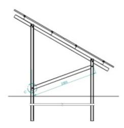
The rear brace in a Stalex free-standing structure, made of an angle bar, is an additional stabilizing element particularly recommended for difficult terrains and demanding projects. By incorporating the rear brace, the structure gains enhanced stability and durability, which is crucial in challenging soil conditions and under greater loads. This solution ensures that the Stalex structure remains reliable and durable even in the toughest ground conditions.
