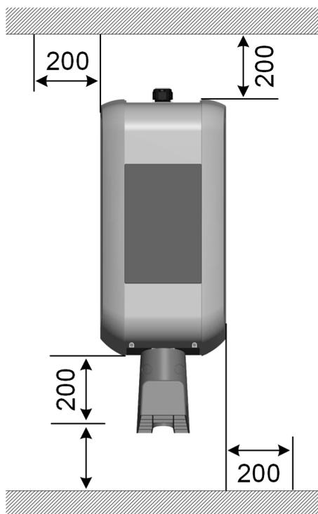
Fig. 6-12: Space requirement, specified in mm
