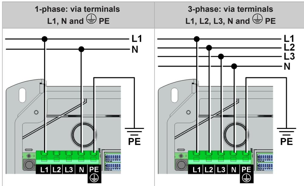
The supply terminals are designed as spring-type terminals. The handling instructions enclosed in the terminal area must be observed.
