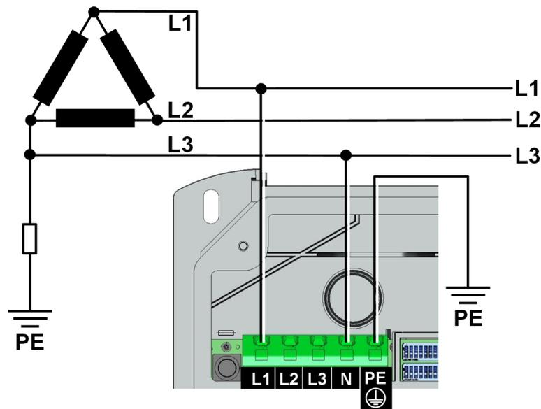
Fig. 7-18: Connection to a three-wire IT system with 230 V
