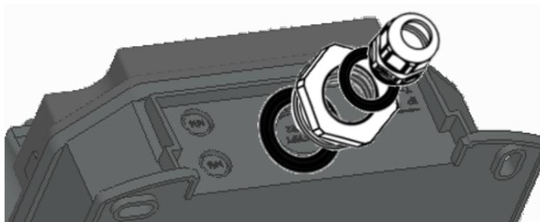
Fig. 7-17: Use of a reducing insert
