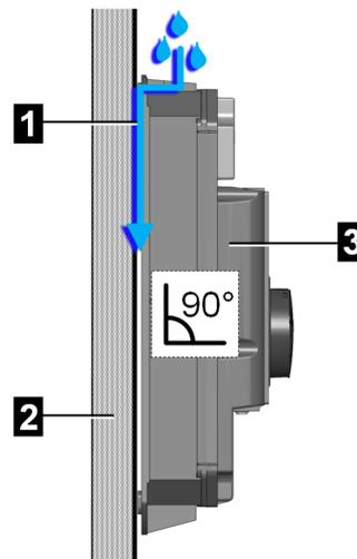
Fig. 6-11: Water drainage
