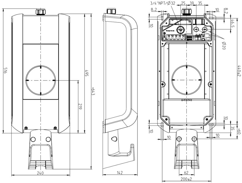
Fig. 13-20: Dimensions in millimeters
