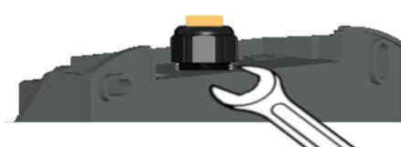
Fig. 6-14: Tighten the cable gland from the back
