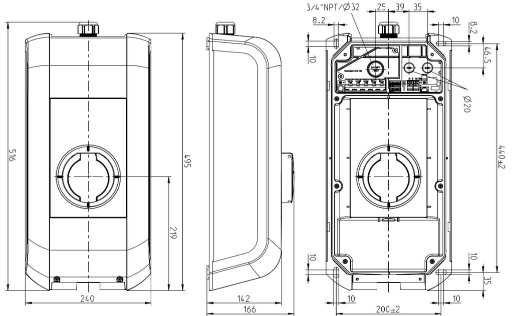
Fig. 13-19: Dimensions in millimeters
