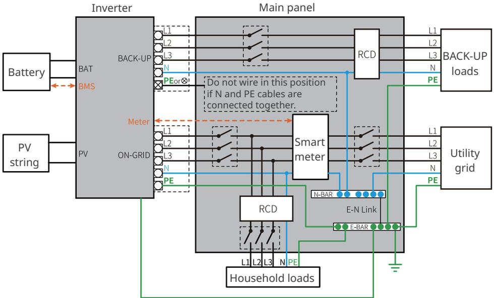
**N and PE cables shall be wired separately in the Main Panel.**
