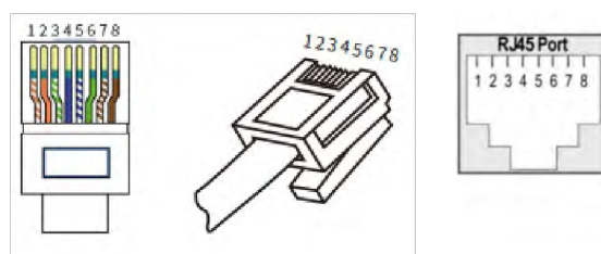
Figure 2-13 "EXT-RS232" port pins
