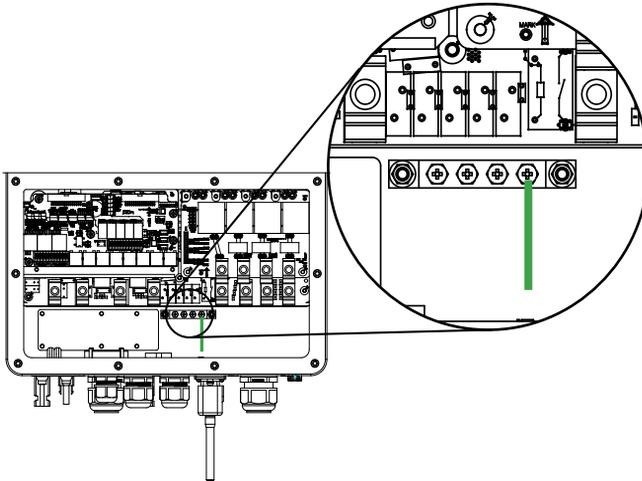
Earth connection(Copper wires)
