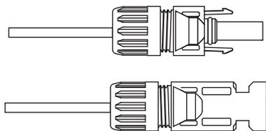
Pic 5.5 connector with cap nut screwed on
