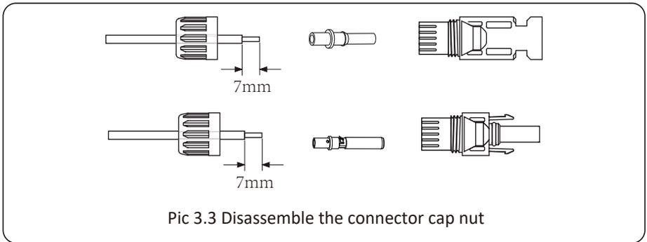
Pic 3.3 Disassemble the connector cap nut
