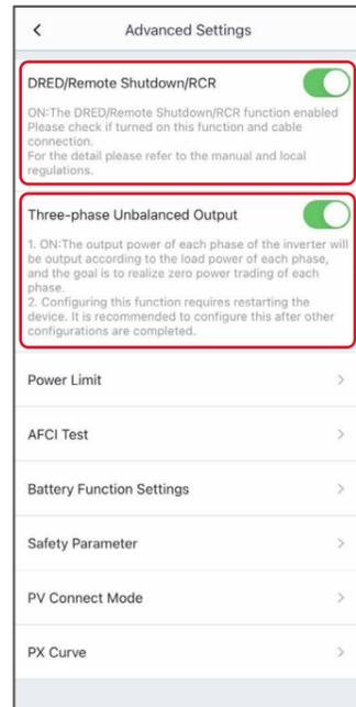
Enable **Three-phase Unbalanced Output** when the utility grid company adopts phase separate billing.
