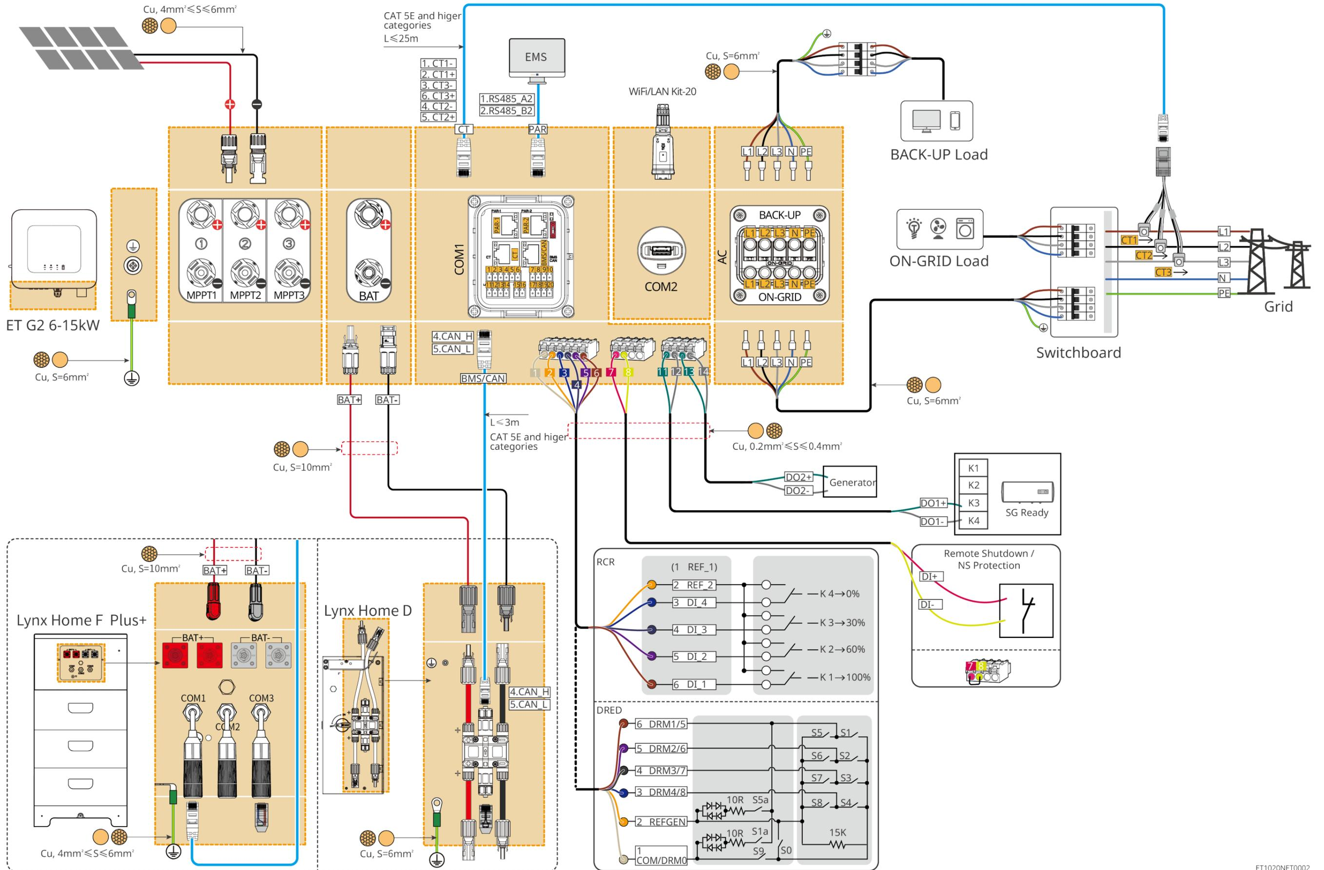
ET G2 6-15kW (parallel connected) + Ezlink3000
