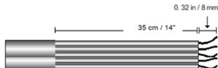
Figure 32: Insulation stripping – AC
