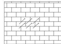
Insert the expansion tubes into the holes and tighten them. Install the bracket with the expansion screws.
