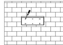
Step2: Match the inverter with wall bracket
