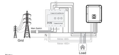
Note: Please be noted that the load/inverter connections and grid connections are illustrated in the figure below. Port 10 is specifically for neutral connection.
