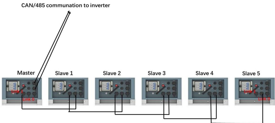
The communication for master/slave string connection shall use a 8pin pin-pin RJ45 cable, connecting from first BMS Link 1 to second BMS Link 0, then from second BMS Link 1 to third BMS link 0(if has), all the way to the last BMS Link 0. The BMS with Link Port 0 EMPTY is defined as the Master string, which further communication with the inverter or upper controller.
