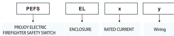
Models: PEFS-EL-x-y. Rated current: x=16/25/32/40/55/40H/50H, Wiring types: y=2/2H/4S/4T/4B/4
