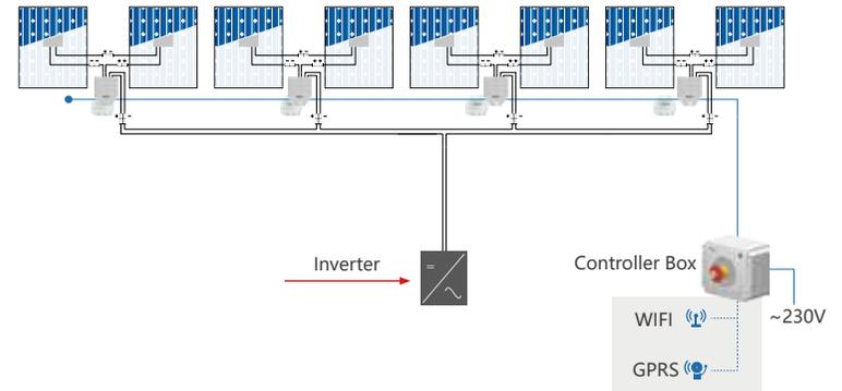
Note: The control box can convert AC 230V to DC 24V, and then control the working status of PEFS.
