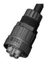
Step 5: Insert seal into body, then tighten the nut, torque 1.5±0.3N·m. The maximum spacing between the nut and the body after tightening is 1.5mm.
