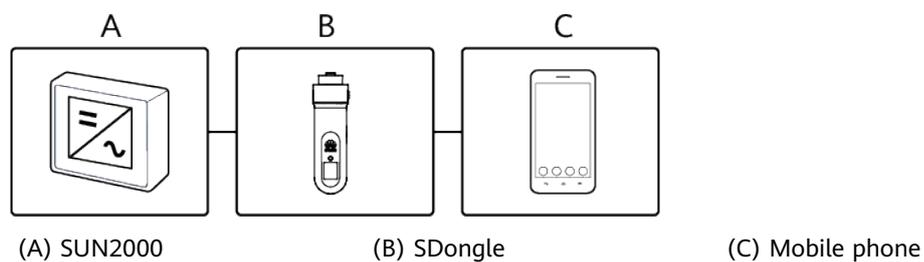
**Figure 7-3** Connection over a USB data cable
