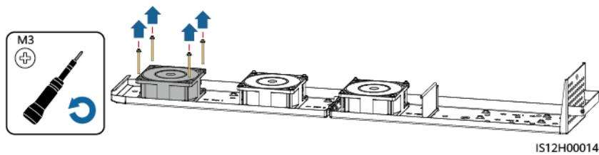
**Step 6** Install the new fan (FAN 1 is used as an example).
