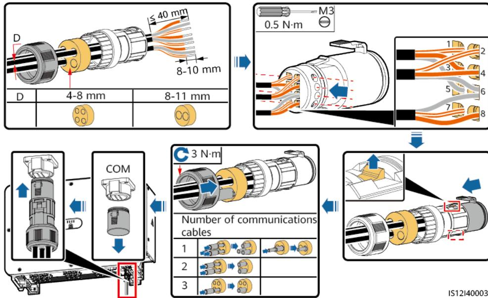
**Figure 5-28** Connecting RS485 communications cables (4–8 mm two-hole or three-hole rubber plug)
