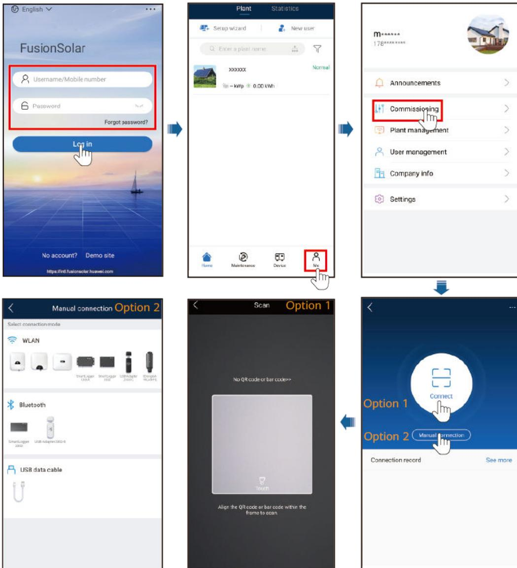
Figure 7-5 Selecting a connection mode (without network access)
