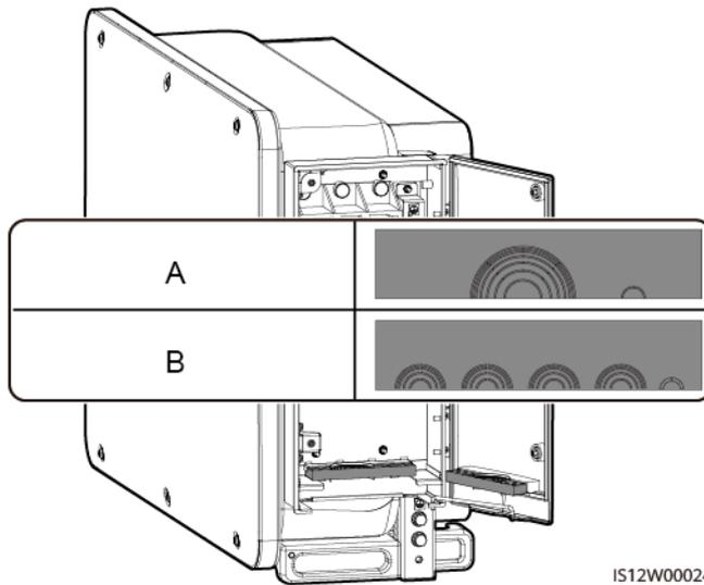
(A) Crimping module for multi-core cables
