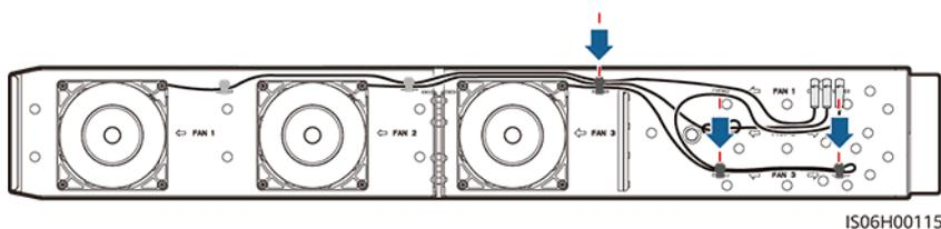
**Step 8** Push the fan tray into the slot until the fan baffle plate aligns with the inverter chassis.
