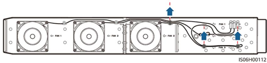
**Step 5** Remove the faulty fan (FAN 1 is used as an example).
