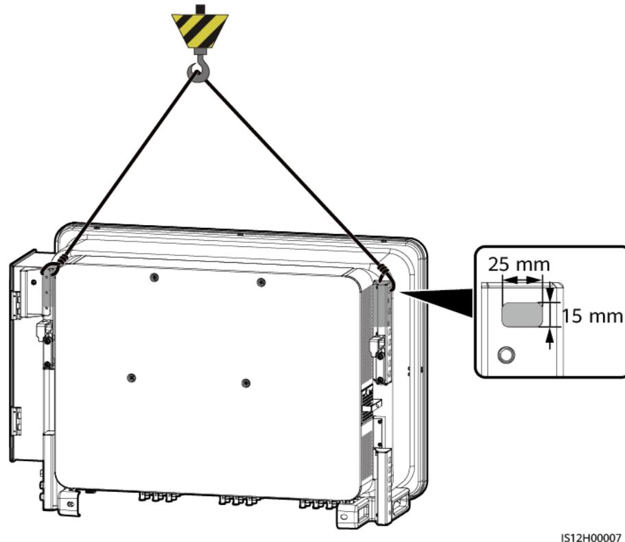
**Step 4** Install the solar inverter on the mounting bracket and align the solar inverter enclosure with the mounting bracket.
