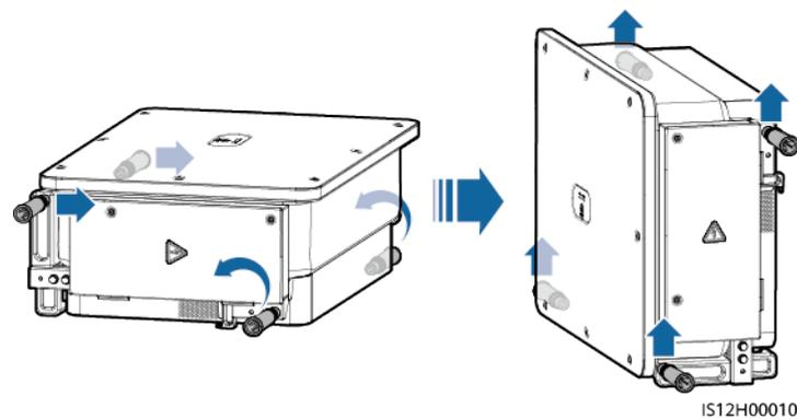
**Step 3** If the installation position is too high to install the solar inverter on the mounting bracket, run a rope that is strong enough to bear the solar inverter through the two lifting eyes, and hoist the solar inverter.
