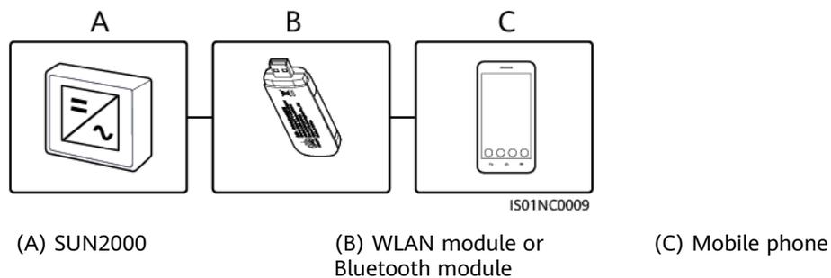
**Figure 7-2** Connection over a Smart Dongle
