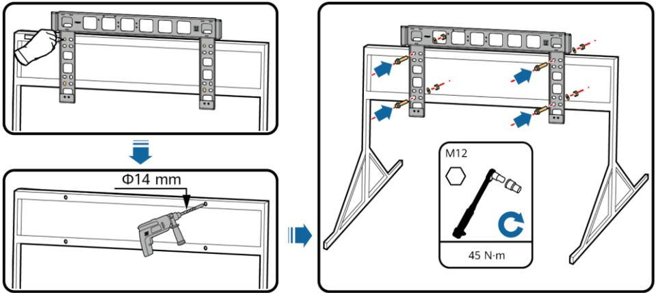
2. Install the solar inverter onto the mounting bracket. 3. Tighten security Torx screws.
