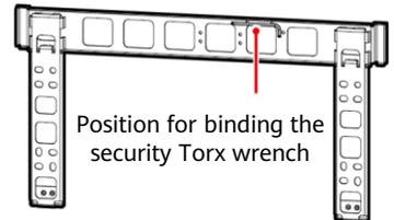
Position for binding the security Torx wrench
